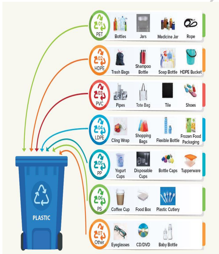
Figure 14 Plastic segregation representation. Source: CPCB Guidelines on Plastic Waste Management
