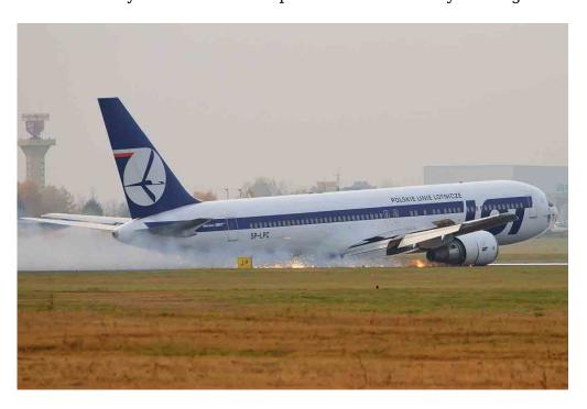
• It also occur when pilots simply forgot to deploy the landing gear and landed aircraft on their belly.
