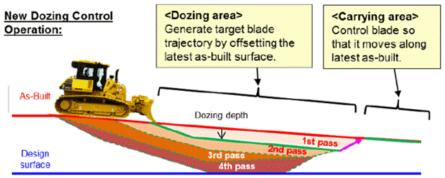
When blade edge approaches design surface, blade automatically follows design surface (same as conventional control)
